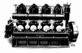
Rear View of Engine, showing exhaust manifold, pump, and service pipes of circulation lubrication
